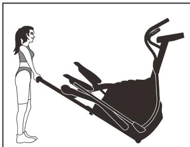
*2. Grasp both Dual Action Handles together and pulling back on handles, tip machine towards you..*
